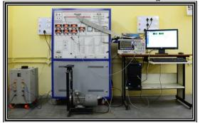
Three Phase Seven-Level Neutral Point Clamped Inverter (Established in Dr. P. Satish Kumar's Research Lab)
