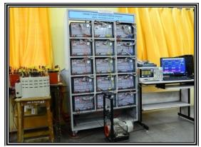
Three Phase Eleven – Level Cascaded H-Bridge Inverter
